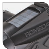
TOP MOUNTED SOLAR PANEL
